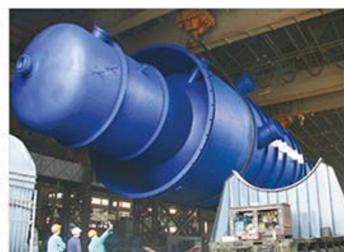
Vacuum Column diameter of 8.5 m, weighing 336 t
