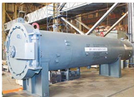
Pig Launcher with a bayonet-type closure DN 1400 mm
