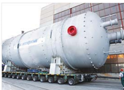
Coke Chamber diameter 7.6 m, weight 210 t
