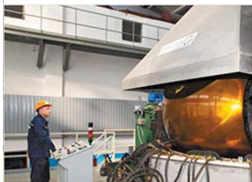
Chromium coating of a ball valve sphere DN 1400 mm
