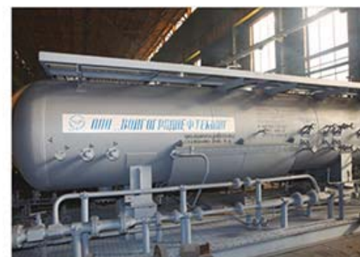
Separator module for NDEG and condensate
