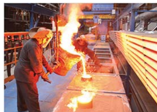
Casting production in a lost foam cast line
