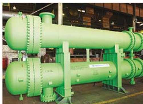
Hydrofining product gas mixture Water Cooler
