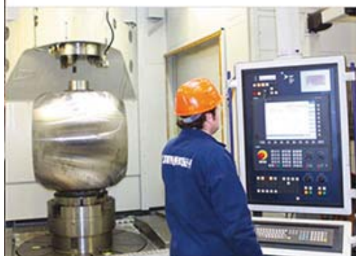
Polishing of a ball valve sphere
