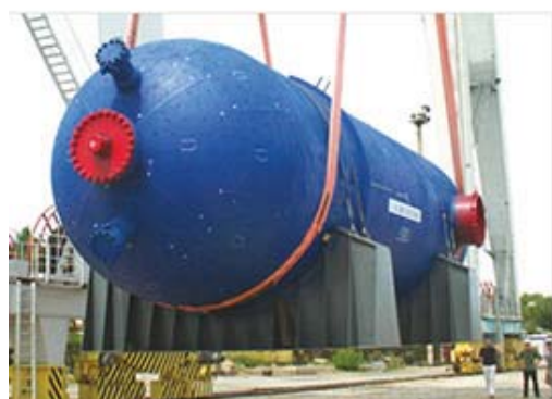
Hydrofining Reactor diameter 4.0 m, wall thickness 180 mm, weight 311 t
